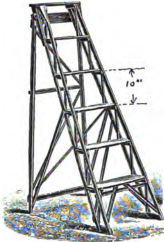
FIG. 46.—Lattice-Work Steps (Section 190).
